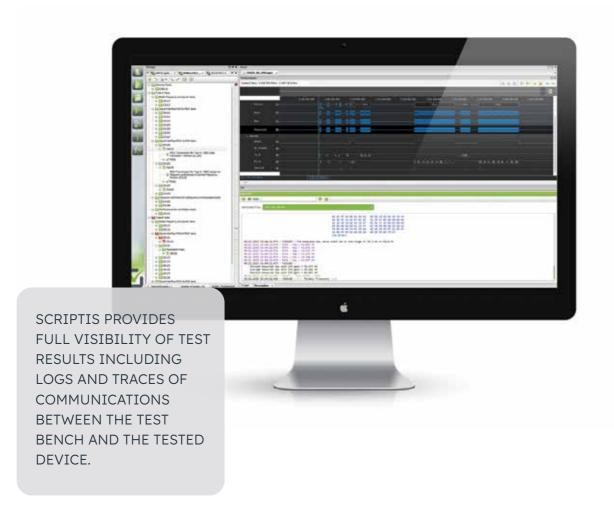
KEOLABS' test suites are used in **SCRIPTIS** testing environment which facilitates testing with automation features such as visual cues and aids for manual testing, or robot integration for fully automated testing. The user controls all the characteristics of the tests such as data exchanged, timing, protocol errors, etc.
