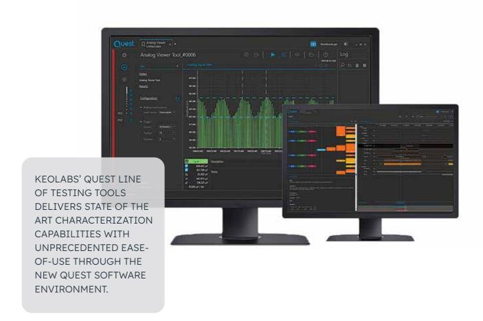
Quest provides characterization tests as preconfigured scenarios. These scenarios control the tester's programmable features to enable single-click access to contactless tests such as waveform analysis and performance profiling.
