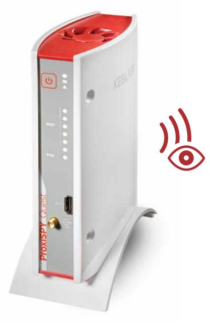
ProxiSPY Quest is the most advanced laboratory tool to trace and analyze contactless communication and troubleshoot the interoperability issues in real-time. Thanks to its cuttingedge technology, ProxiSPY Quest provides an efficient and complete analysis, from the analog to the application layer. It can be used in transport, mobile, and contactless payment fields to analyze and debug new products and ensure inter-device compatibility.
