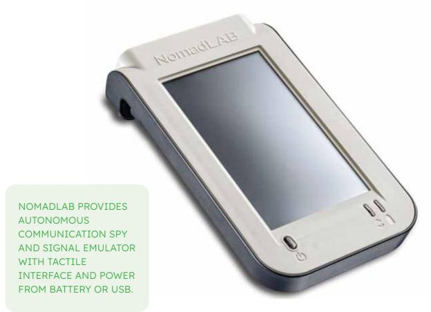
It is equally adapted to application testing in a lab or field environment, providing communication spy and analysis for NFC, ISO/IEC 14443 A/B card signals, FeliCa, ISO/IEC 7816, SWP (HCI/ SHDLC), emulation of ISO/IEC 7816, and ISO/IEC 14443 card signals for active testing of card readers.
